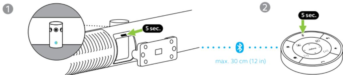
To pair, the remote control must be within 30 centimeters (12 inches) of the Jabra PanaCast 50.
