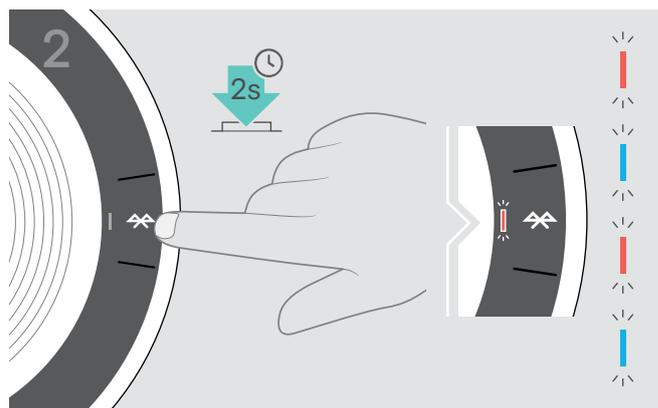
▶ Press and hold the Bluetooth button until the LED flashes blue and red. The speakerphone is in pairing mode.
