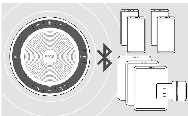
The speakerphone can save up to eight paired Bluetooth devices. If you pair the speakerphone with a ninth Bluetooth device, the saved connection profile of the least recently used device will be overwritten. If you want to re-establish a connection with this device, you have to pair the speakerphone again.
