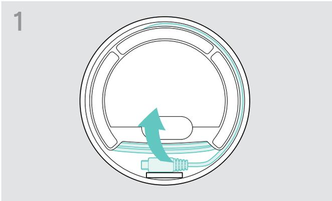
▶ Release the USB plug from the holder and unwind the cable.
