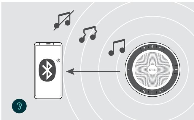
If you leave the Bluetooth transmission range, the audio quality deteriorates first and later connected devices will be disconnected.
