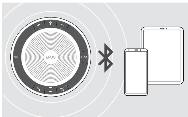
The Speakerphone can be wirelessly connected to two devices at the same time.
