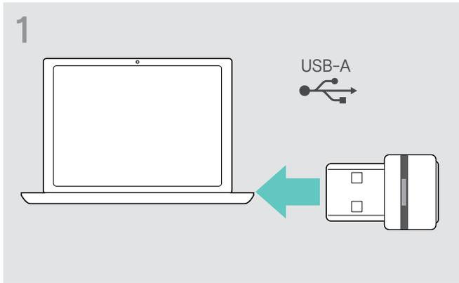
▷ Plug the dongle into the USB port of your computer.
