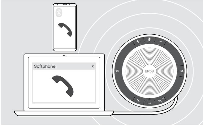
You can use the Speakerphone with up to three connected devices, one connected via USB and two via Bluetooth.
