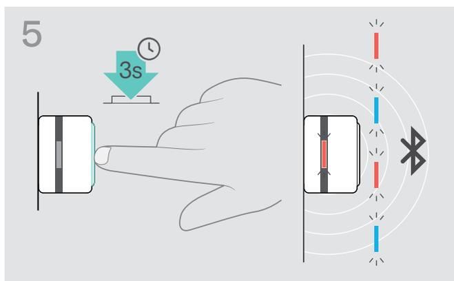
▶ Press and hold the dongle's button until the LED flashes blue and red. The dongle is in pairing mode.
