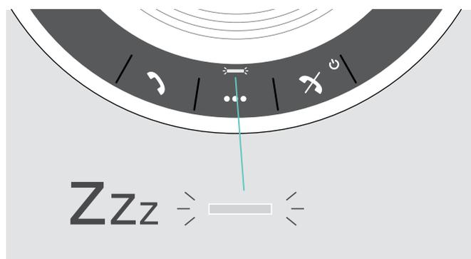
While in standby the activity LED is dimmed and all other LEDs are off.
