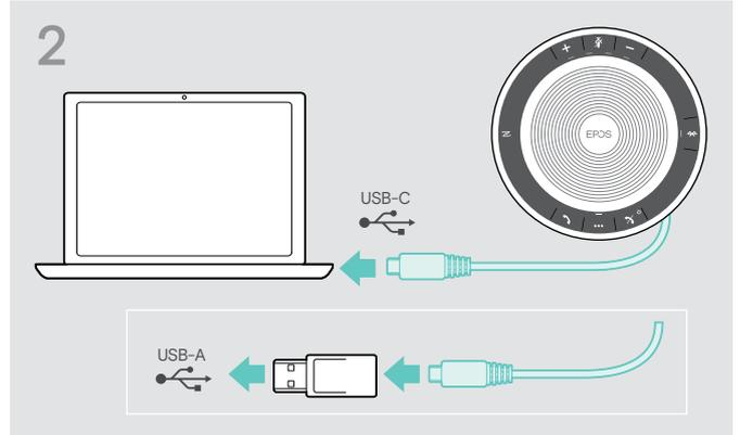
▶ Connect the USB connector directly to a USB-C port or to a USB-A port using the included adapter.
