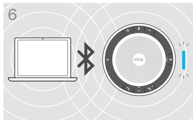
Once the speakerphone is paired with the dongle, the LED lights up blue.
