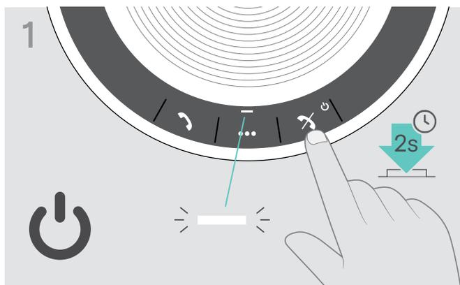
▶ Press and hold the Power on/off button to turn on the speakerphone. The LED lights up white.
