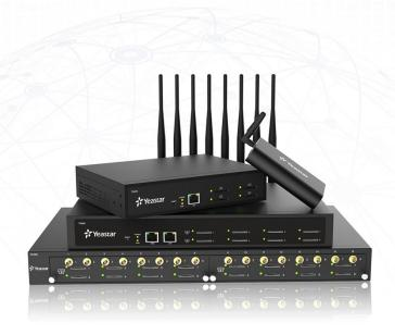
Yeastar TG is a series of VoIP 4G gateway connecting 4G LTE network to VoIP network directly and can support two-way communication: 4G to VoIP or VoIP to 4G. It is the best 4G trunking solution for IP-based telephone systems, the best fallback solution in case of landlines outages, and also the best alternative for areas with limited landline or SIP connection.
